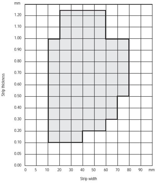
When ordering hot-dip galvanized cable steel strip, please state if the thickness includes zinc coating.
